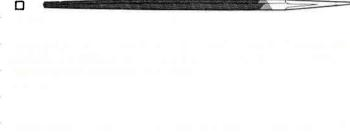
Threesquare For filing out sharp corners and internal angles. Double cut on all three sides. Tapers slightly towards point.
